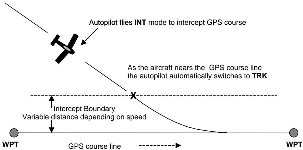
In both the **CRS** and **INT** modes the ground track to be followed may be selected by the pilot, using either the L/R switch or the PCS steering mode of operation
