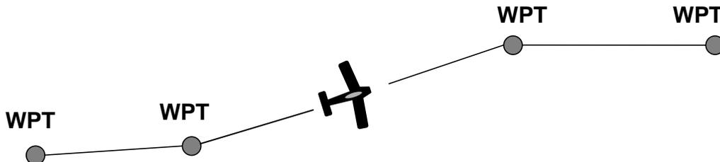
**2. Course mode (CRS)** – provides vector navigation as illustrated below. **CRS** also allows tracking an autopilot-selected course when the host GPS route function is not in use. **CRS** mode uses the GPS signal to provide the aircraft groundtrack. This mode can be useful for avoiding restricted airspace, weather and oncoming air traffic.
