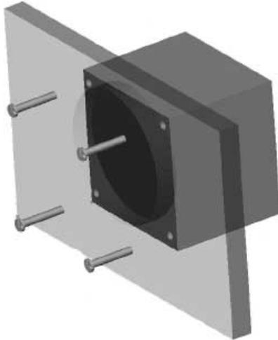
The EZ Pilot control head mounts from the rear side of the instrument panel. It is held in place by 4 ea. Number 6 screws. When mounted, the visible area is contained within a standard 3-1/8 inch instrument cutout.
