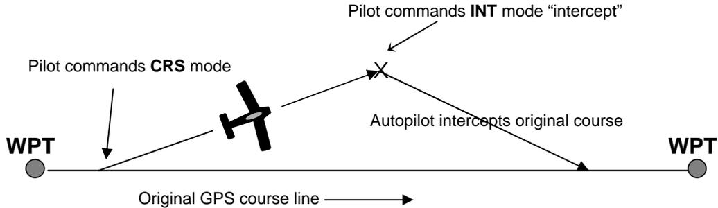
**3. Intercept mode (INT)** – used to intercept a predefined GPS desired track (**DTK**) as illustrated below. The **INT** mode also uses the GPS signal to provide the aircraft groundtrack. This mode is useful to regain the original flight plan track after circumnavigating the previously mentioned flight obstacles.
