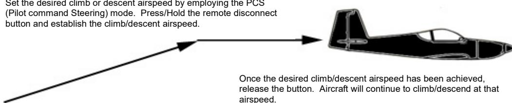
Once the desired climb/descent airspeed has been achieved, release the button. Aircraft will continue to climb/descent at that airspeed.
