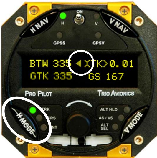
The image shows the Pro Pilot display with a good GPS signal present, and flight plan entered. Note that the "H" (H NAV) LED is illuminated.
