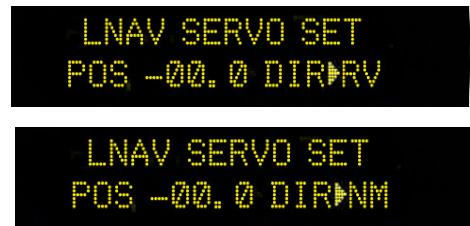
If the elevators or ailerons do not move in the proper direction, the jumper plug inside the respective servo must be removed using the procedure on the next page.
