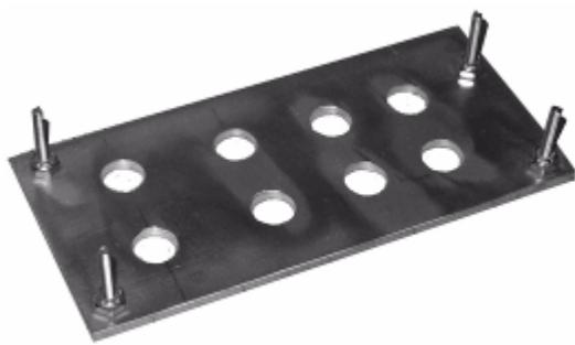
When mounting the servo, be careful not to drill mounting holes into critical load bearing members. It may be best to construct a mounting plate, place and bond machine screws so that they will interface with the case mounting holes, and then secure the assembly into place. For a composite aircraft installation, the bottom of the plate (shown) should be floxed and the holes in the plate filled with flox before applying fiberglass layers over it to secure it to the fiberglass structure.
