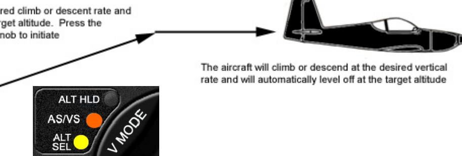
The aircraft will climb or descend at the desired vertical rate and will automatically level off at the target altitude
