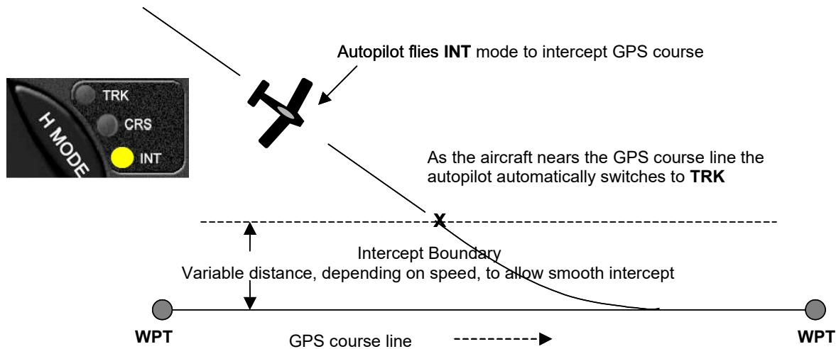
In both the **CRS** and **INT** mode, the ground track heading may be changed by rotating the encoder knob or using the **PCS** steering mode of operation.
