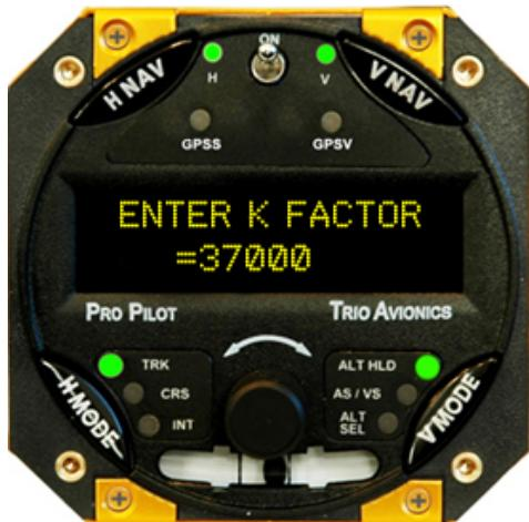
The calibration may be tested by filling the tanks and flying the aircraft until the remaining fuel is down to 25% or less. This will assure a large enough sample to determine accuracy. If it appears that the fuel remaining is not the correct amount (it will likely be very close) The **K FACTOR** may then be adjusted up or down to improve the accuracy.
