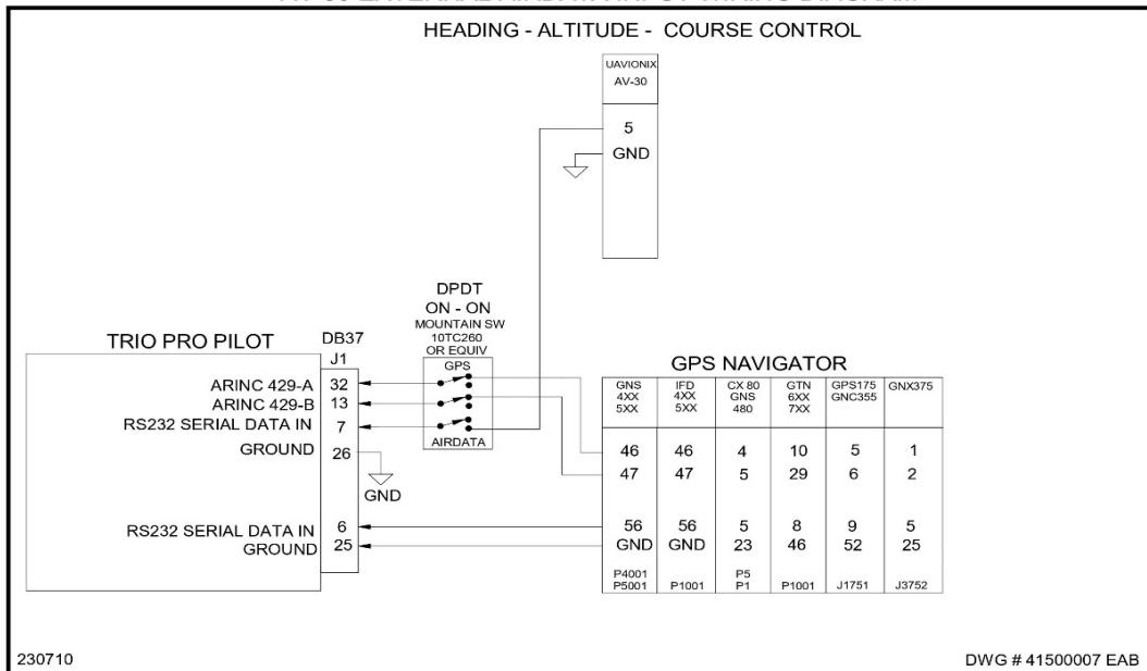
EXTERNAL AIRDATA INPUT WIRING DIAGRAM
