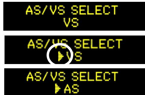
The **AS/VS SELECT** procedure is complete and the encoder can now be used to select another menu screen.
