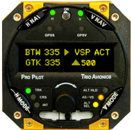
To work properly, the Pro Pilot must start with accurate altitude information. Once the pilot has adjusted the baro setting on the aircraft altimeter, the **ALTITUDE** setting in the Pro Pilot may be easily adjusted to agree with the aircraft altimeter by repeatedly pressing the **V MODE** button to display the **ALTITUDE SET** screen and changing the altitude setting by rotating the encoder knob.
