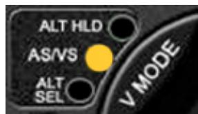
If the encoder knob is now pressed, the **ALT HLD** LED will turn off and the **AS/VS** LED will illuminate and the display screen will show **VS ACT** (Vertical Speed Active). The aircraft will then begin a climb at the selected rate. (The **ALT SEL** LED may also be illuminated if there is an active preselected altitude)
