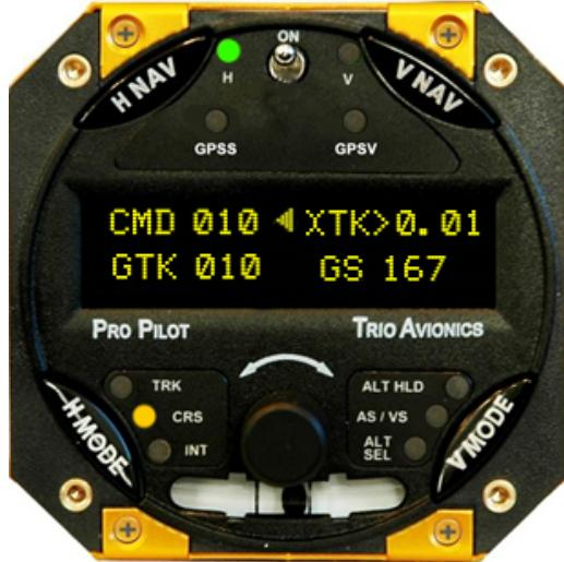
desired **CRS** is 040 degrees so the **ENCODER** is turned clockwise until 040 is displayed as the **CRS** value. The Pro Pilot turns the airplane until both the commanded track (**CMD**) and the ground track (**GTK**) are the same (**040**).
