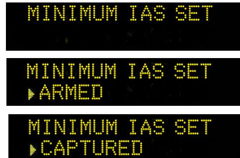
The **MINIMUM AS SET** procedure is complete and the encoder can now be used to select another menu screen.
