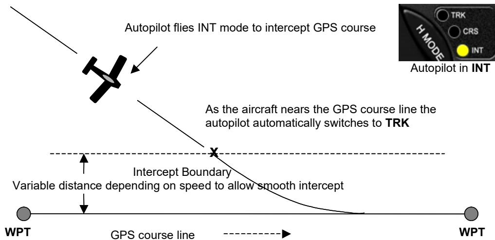
The automatic transition from the **INT** mode to the **TRK** mode is a function of the **XTK** (crossover error) magnitude, which is an index of the difference between the original course line and the position offset from the course line.
