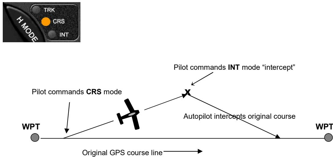
**Hint:** An alternative method of using the **CRS** mode is in conjunction with the Pilot Controlled Steering (PCS) mode of operation (see pages 30 & 31).
