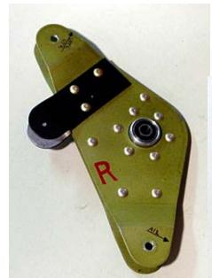
(Left) Tabs have been rounded at the tips and riveted in place. The next step is to drill the hole for the bolt which captures the bearing to final size. (Below)
