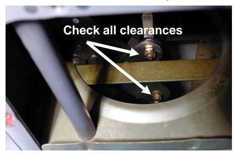
\* Aileron control travel limits are defined by Van's. Limits are set by mechanical stops that are attached to the airframe. Following installation, verify aileron travel is limited by the mechanical stops on the airframe, NOT BY THE ROTATIONAL LIMITS OF THE SERVO. If you do not have experience working with aircraft control rigging, please seek the advice of an EAA Technical Counselor or someone else with appropriate skills and experience.
