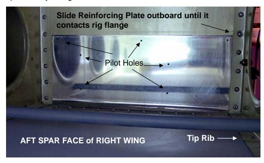
Your reinforcement plate may have up to nine large (.375") holes drilled (as shown below) in it to allow the servo to mount flush against the reinforcement plate. **ONLY THE SEVEN SMALL PILOT HOLES WILL BE DRILLED THROUGH THE SPAR**. Four that attach the servo and three across the top of the reinforcement plate. The three across the top of the plate also secures the reinforcement angle on the front side of the spar. (See images on next page)
