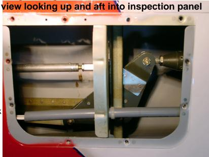
**Step 2:** Drill out the two rivets located on the CONTROL STICK END of the bell crank. Align the servo push tube mounting tabs to the bellcrank as shown below. Align the tabs on the CONTROL STICK END of the bellcrank with the tabs extending out from the long side (hypotenuse) of the triangle.
