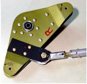
**Step 4:** With the servo hub centered (crank pin in the hub facing straight up), install the crank arm straight up as shown below.
