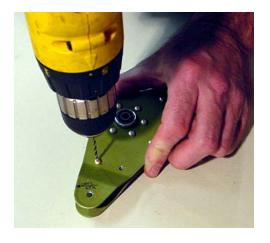
Using bellcrank as drilling template, align and drill tabs.
