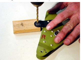
Use a ½" block, inserted between the tabs, to drill the bearing hole to final size. Try to drill this as "square" as possible. A drill press will help if available.
