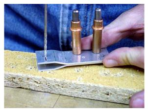
Remove the tabs from bellcrank, cleco them together, and pilot drill the bearing hole.
