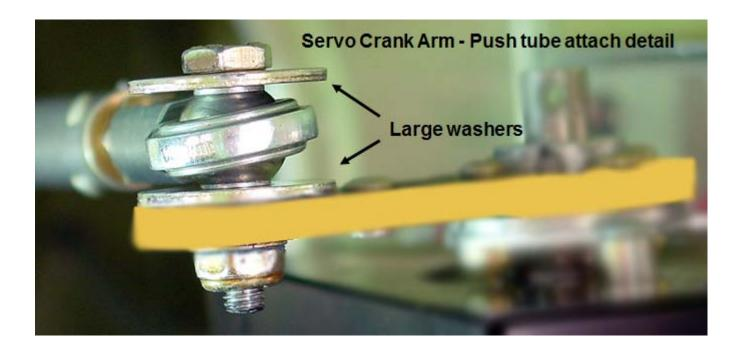
**Step 10:** Attach servo push/pull tube to aileron bell crank. Note: Your kit contains hardware for attaching the push/pull tube to the bell crank. We have provided a variety of washers (spacers) for the installation.
